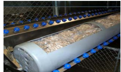
Sliced packaged meat which is in place and ready to be treated by a high-pressure processing machine
